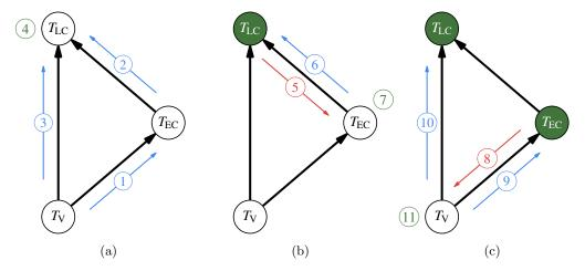
FIG. 3: Example of dependency resolution when a new Model is uploaded to the processing pipeline. Black arrows indicate upstream dependencies while blue and red arrows represent upstream and downstream resolution, respectively. (a) Upstream resolution begins from  $T_{\rm V}-M$  and leads to  $T_{\rm LC}-M$  being run. (b) Downstream resolution begins from  $T_{\rm LC}-M$  and leads to  $T_{\rm EC}-M$  and leads to  $T_{\rm V}-M$  being run.
