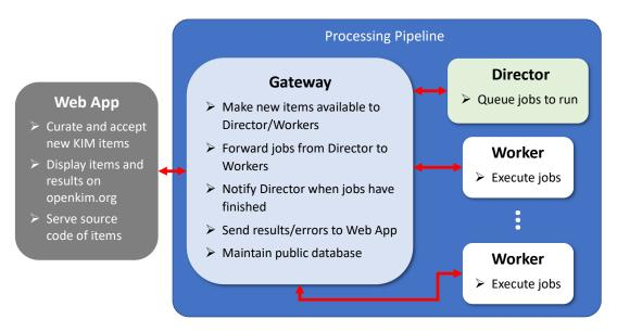
FIG. 1: Abstract architecture of the pipeline and the responsibilities of each component. Arrows indicate connectivity.
