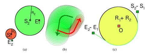
Figure B.1: Two robot problem. (a) Robot 1, of radius  $R_1$ , must start at  $\vec{S}_1$  and end at  $\vec{E}_1$ . Robot 2, or radius  $R_2$ , starts at  $\vec{S}_2$  and ends at  $\vec{S}_1$ . The robots must not collide at any time, and must minimize  $\frac{\gamma}{2}(\int_0^T (\dot{\vec{r}}_1(t) + \dot{\vec{r}}_2(t))^2 dt)$ , where  $\vec{r}_i(t)$  is the position of robot a at time t. (b) Subsampling of the exact solution. (c) The problem in the reference frame of robot 1.
